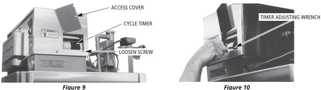
The cycle timer (*Figure 9*) makes one complete revolution (one dishwasher cycle) in 90 seconds. It consists of seven cams, four of which can be adjusted. These cams actuate switches which control various machine functions. A degree marker is located at the right end of the timer and corresponding notches on each cam are marked off in five degree increments. Every four degrees of rotation equals one second.
