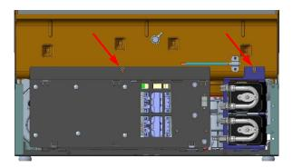
► Lower control board bracket and chemical pump bracket to allow access to terminal block 1TB.
