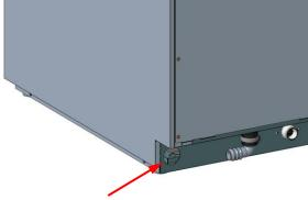
► Install 1" trade size conduit or cable and fitting. Leave at least four feet of electrical line between wall connection and machine. This allows machine to be pulled away from wall for cleaning and/or servicing.
